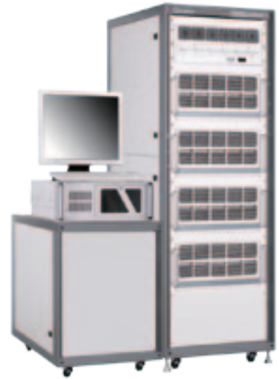
17011 Charge/Discharge Test System
